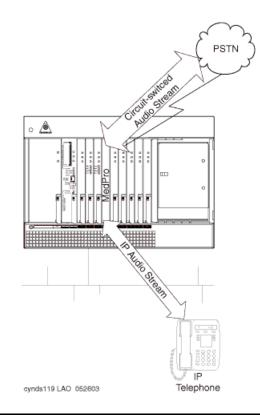
To do the job, a media processing circuit pack has a set of DSP resources. These resources are deployed dynamically and flexibly to any of a number of tasks, including:
